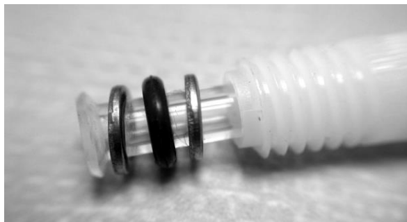
Flanged Connector: Requires Flat Black Washer On ports A and C and for any others that leak
